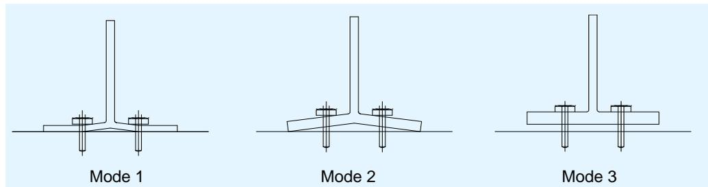
**Figure 1.2 Behaviour modes of an equivalent T-stub**
