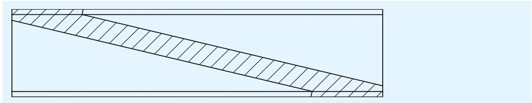
Figure 3.1 Fabrication of haunch cuttings
